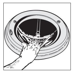
6 Check the folds in the door seal for any small articles such as buttons or nails which may be lodged there.
